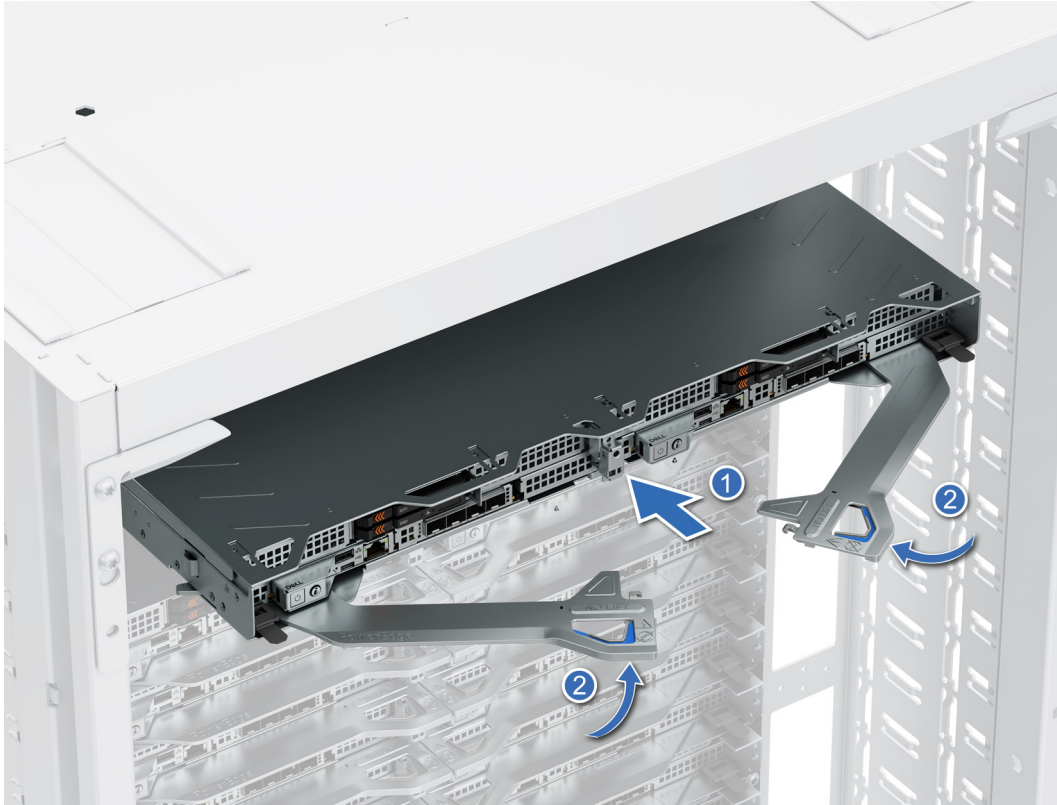
Figure 17. Server installation in the rack
