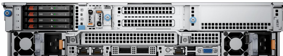
Figure 12. Rear view of the system with 4 x EDSFF E3.S rear drive module
