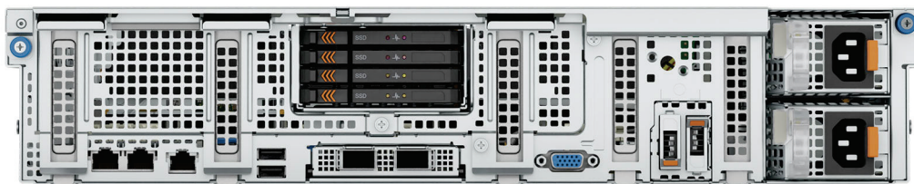
Figure 12. 5 x PCIe Low-Profile Slots + 4 x E3.S NVMe Drives
