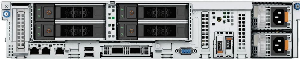
Figure 4. 2 x PCIe Low-Profile Slots + 4 x 3.5-inch SAS/SATA Drives with 1 CPU
