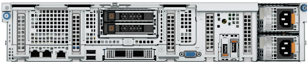
Figure 8. 3 x PCIe Low-Profile Slots + 2 x 2.5-inch NVMe Drives with 1 CPU
