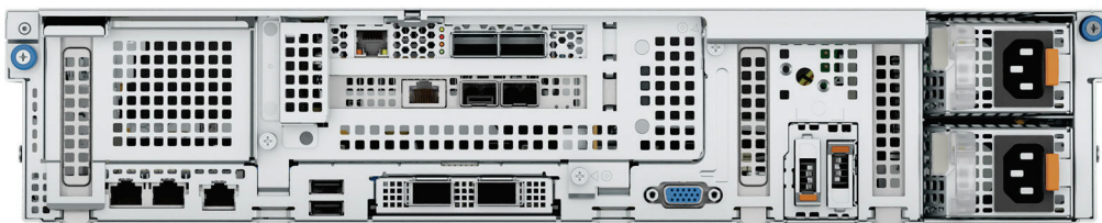
Figure 9. 3 x PCIe Low-Profile Slots + 2 x PCIe FH/FL Slots
