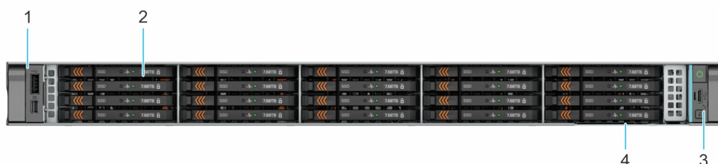
Figure 6. Front view of 20 x EDSFF E3.S drive system
