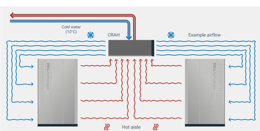
Traditional air cooling relies on a hot aisle/cold aisle layout: cold air cools the servers, exits as warm air, and is recooled by computer room air handlers (CRAHs) using ~10°C facility water before cycling back.
