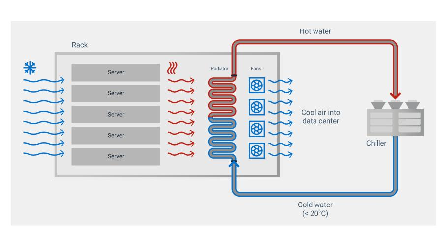
An RDHx delivers facility water directly to the rack, using coils and fans to cool hot server exhaust. It enables higher water temps (~20°C vs. ~10°C) and greater compute density per rack.
