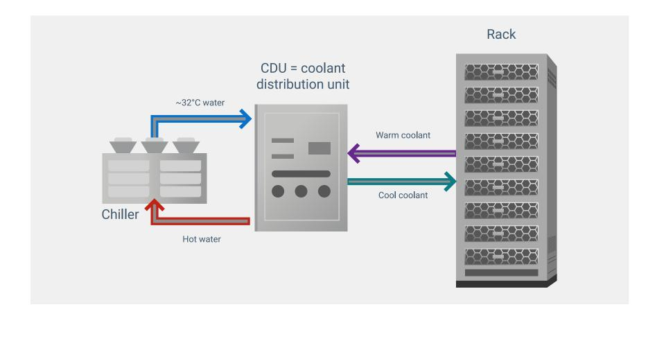
Hybrid direct liquid cooling (DLC) uses cold plates inside the server chassis to cool hot components like CPUs and GPUs, while air handles the rest. A coolant distribution unit (CDU) controls flow and temperature of the liquid, enabling efficient cooling with ~32°C facility water.
