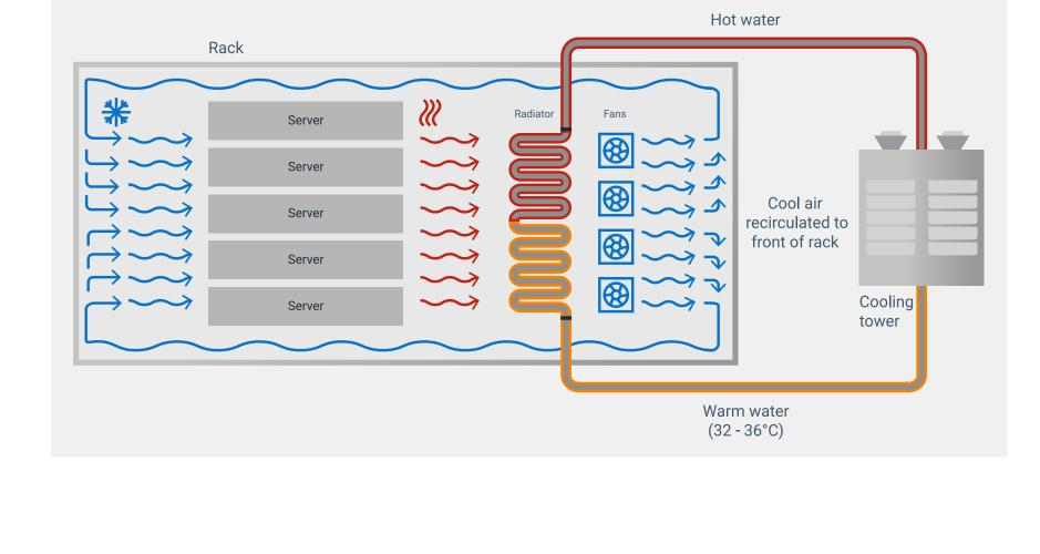
The Dell PowerCool Enclosed RDHx is a fully enclosed, rack-scale solution that cools all components using warm facility water (~32–36°C). By sealing and recirculating air within the rack, it boosts efficiency and eliminates the need for energy-intensive facility chillers.
