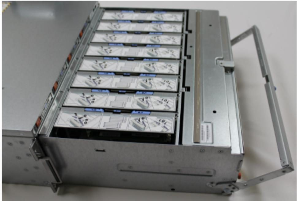
**Figure 104** Releasing a memory riser
