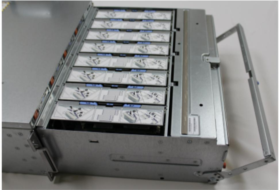
**Figure 88** Releasing a memory riser
