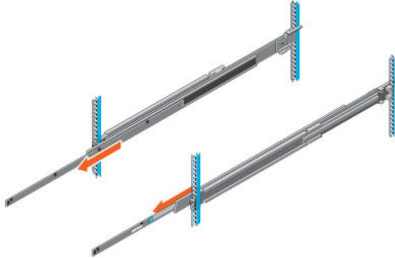
2. Locate the rear rail standoff on each side of the system. Position the system above the rails and lower the rear rail standoffs into the rear J-slots on the slide assemblies.
