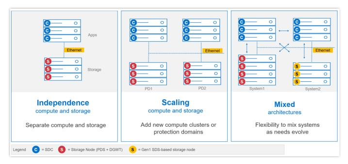
The functional character of a node, its personality, is determined primarily by the installation/presence of software services running on the node. However, PowerFlex nodes are configured and purchased as either "storage" or "compute" nodes. This reflects the type and quantity of resources in the node, ensuring that resources align with
