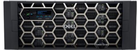
PowerScale A3100 builds on the A3000 platform to deliver a dense archive solution — now with upgraded compute, DDR5 DRAM, and improved thermal design for better performance under scale. Storing up to 1.9 PB per chassis, and supporting future HAMR HDDs as well, the A3100 combines long-term retention efficiency with the agility needed for active archive scenarios. Ideal for high-volume datasets, it accelerates retrieval of cold data to support retraining, versioning, and compliance workflows.
