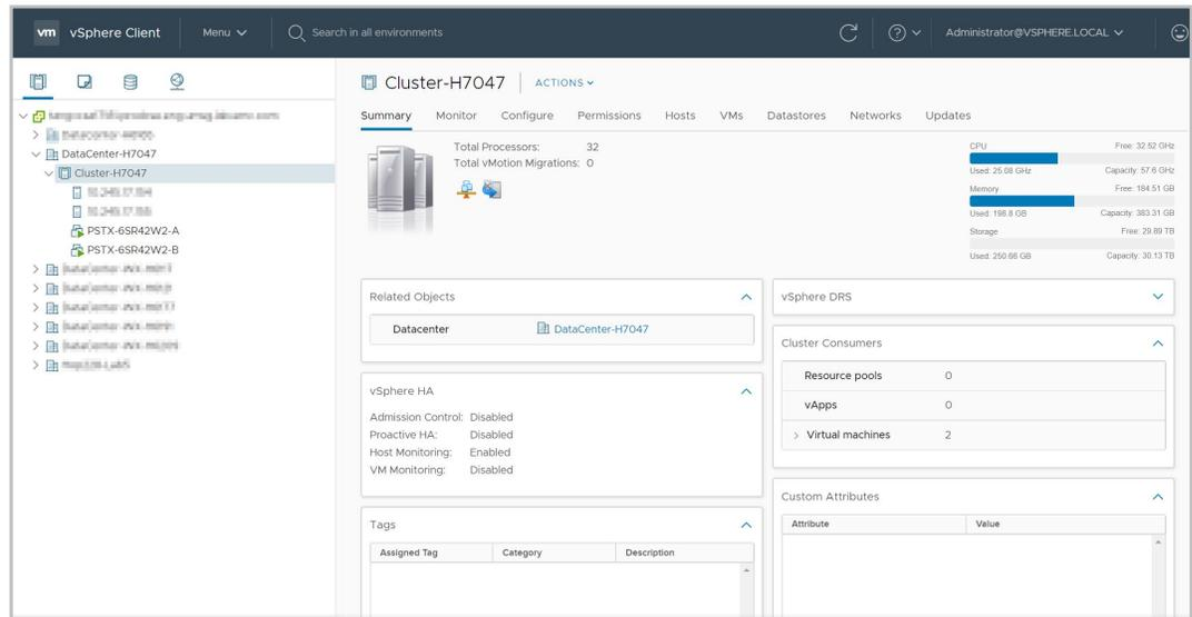
**Figure 28. PowerStore X model objects in vSphere**
