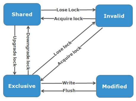
Figure 10. OneFS cache coherency state diagram
