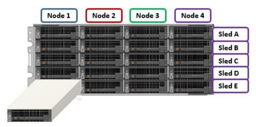
Figure 18. Gen6 platform chassis front view showing drive sleds
