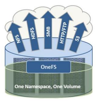
Figure 5. Single file system with multiple access protocols
