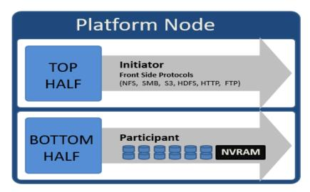
Figure 6. Model of node components involved in I/O
