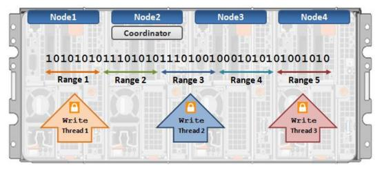
Figure 14. Multi-threaded IO writer
