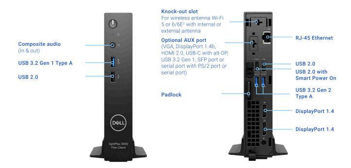
Built with Intel® Celeron and Pentium Quad Core™ processors (Celeron N5105 2GHz/2.9GHz and Pentium N6005 2GHz/3.3GHz Up to three 4K displays @60Hz5 with 2 native DisplayPort™ 1.4 interfaces and optional DP 1.4b, HDMI 2.0 or USB-C with alt-DP or VGA
