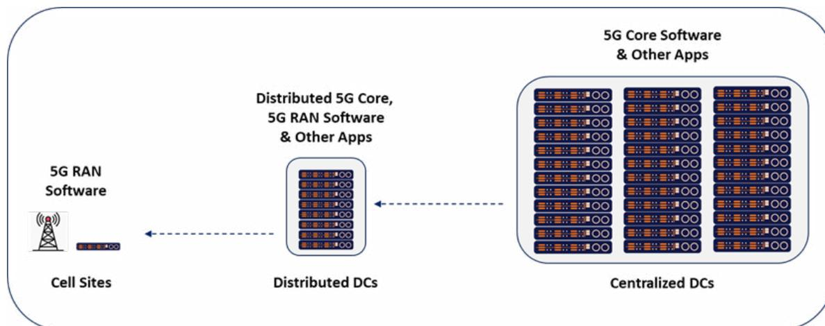
**Figure 1. Example in 5G Implementations of CSPs' Increasing Distribution of Bare Metal Hardware in Their Infrastructures for New Services and Applications**
