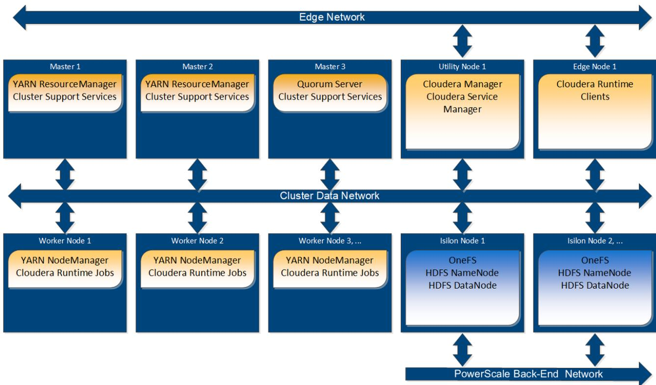
**Figure 2. Node-level architecture with PowerScale storage**
