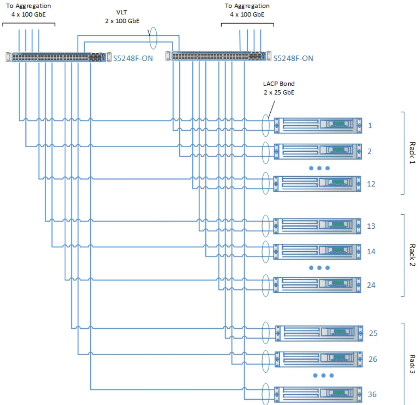
**Figure 6. 25 GbE single pod networking equipment**
