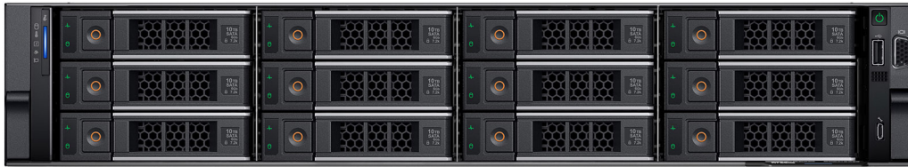
Figure 4. Front view of 12 x 3.5-inch drive system
