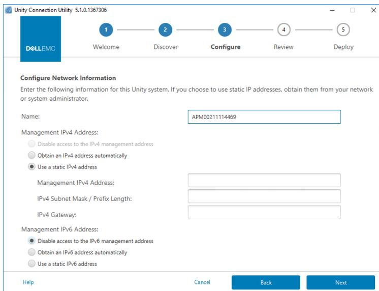
Figure 3 Unity Connection Utility IP Configuration
