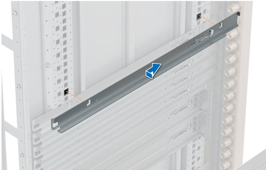
Figure 51. Installing the static rails in IR7000 rack before installing M7725 system
