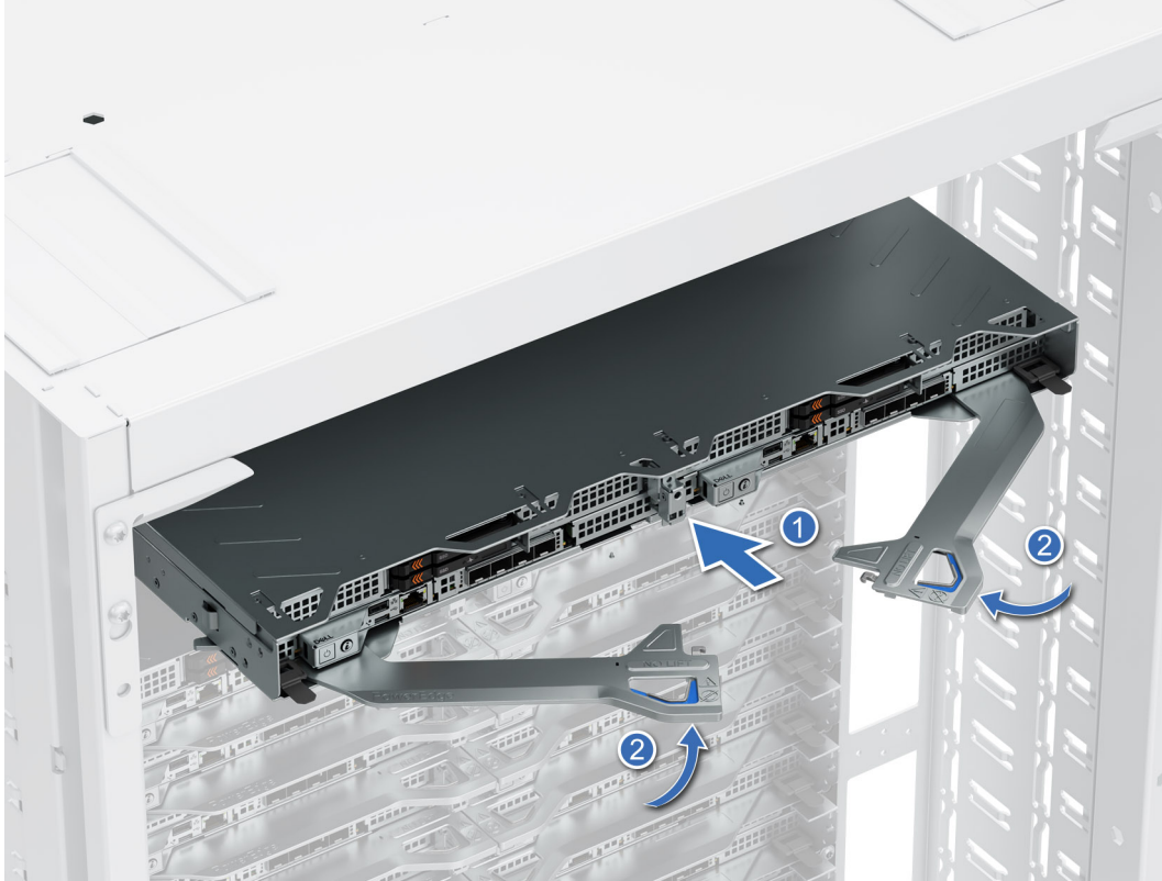
Figure 14. Server installation in the rack
