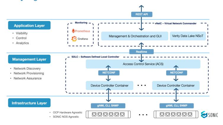
Verity uses three separate virtual machines (VMs) that split application, control, and observability duties. The **Virtual Network Commander (vNetC)** VM runs the web-based GUI and is responsible for all application-layer services for network visibility, orchestration, analytics, and the northbound RESTful API.
