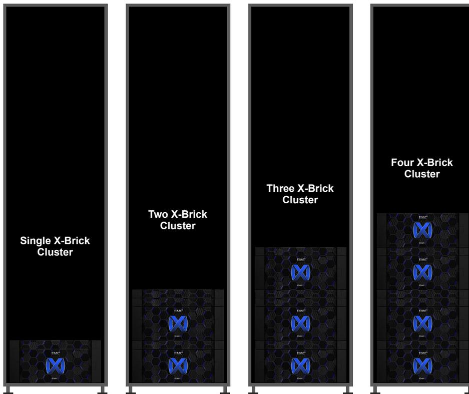
Figure 2. System Configurations as Single and Multiple X-Brick Clusters
