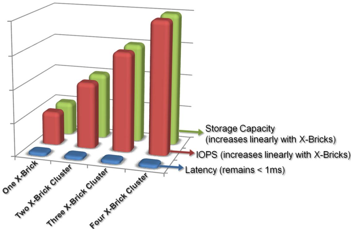
Figure 20. Linear Performance Scalability with Consistent Low Latency
