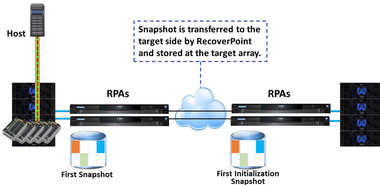
Figure 26. RecoverPoint "Snap and Replicate" Option—Initial Replication
