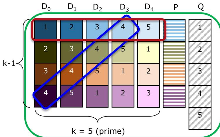
Figure 17. Row and Diagonal Parity
