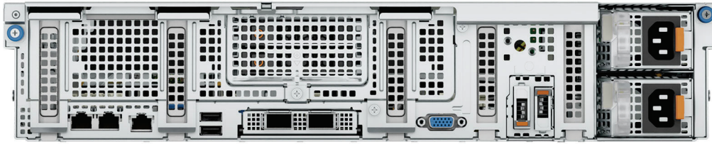
Figure 6. 3 x PCIe Low-Profile Slots with 1 CPU
