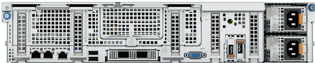
Figure 5. 5 x PCIe Low-Profile Slots
