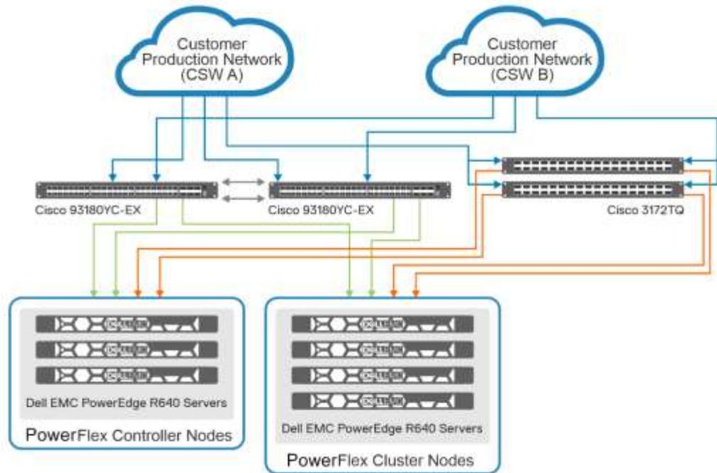
**Figure 16. Solution architecture**
