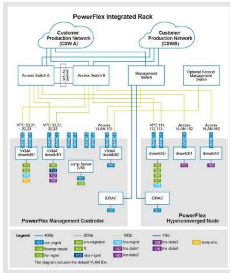
Figure 17. Virtual networking in PowerFlex rack
