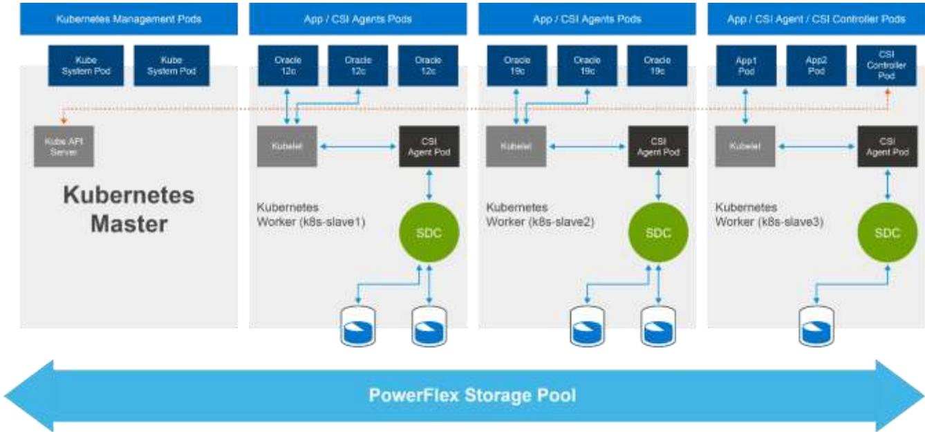
Figure 4. PowerFlex and Kubernetes architecture with the CSI driver
