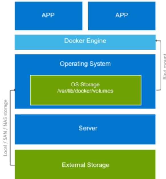
Figure 7. Linux bind mounts
