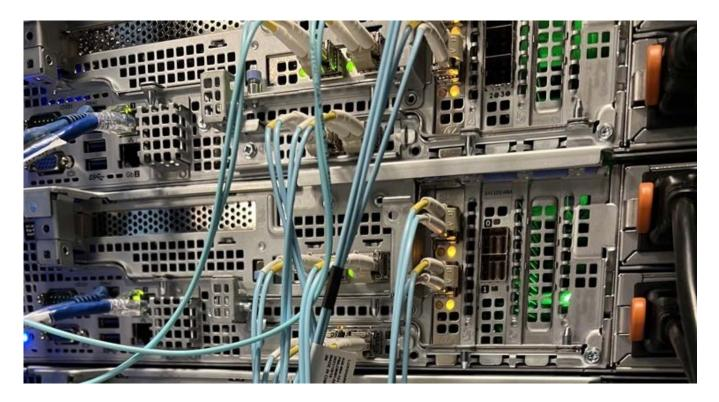
To get started, the PowerProtect appliance must be in a rack, cabled to the network switch, and powered on. If those steps are complete, attach the service computer to the appliance, and set up a static IP address and subnet on the computer. Ping the management IP address, 192.168.100.100, to verify it's reachable. Open a browser window, enter https://192.168.100.100, and connect to the appliance to display the configuration login screen.
